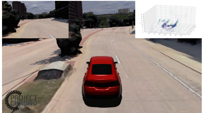
Fig. 2. A sedan drives through a simulated world. The views from a forward-facing (main image) and rear-facing (top-left) camera are rendered with CHRONO::Sensor along with the view from a lidar (top-right)
