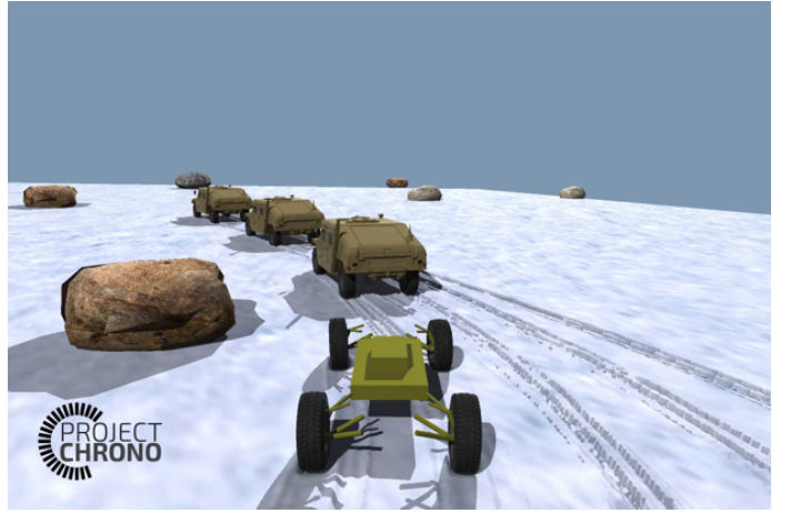
Fig. 5. With the final policy learned, a convoy of four vehicles navigates a field of obstacles. The fourth vehicle is displayed without a chassis asset to showcase suspension motion as it moves over ruts. The deformable soil used in this case is given a snow texture as it is a relatively soft soil.
