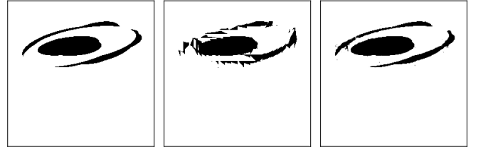
Fig. 1. A selected sample demonstrating network output. Left: ground truth image, constructed by superimposing randomized shapes; middle: input image to network, created by mapping the ground-truth data to a mesh and performing a PLIC reconstruction; right: network reconstruction.
